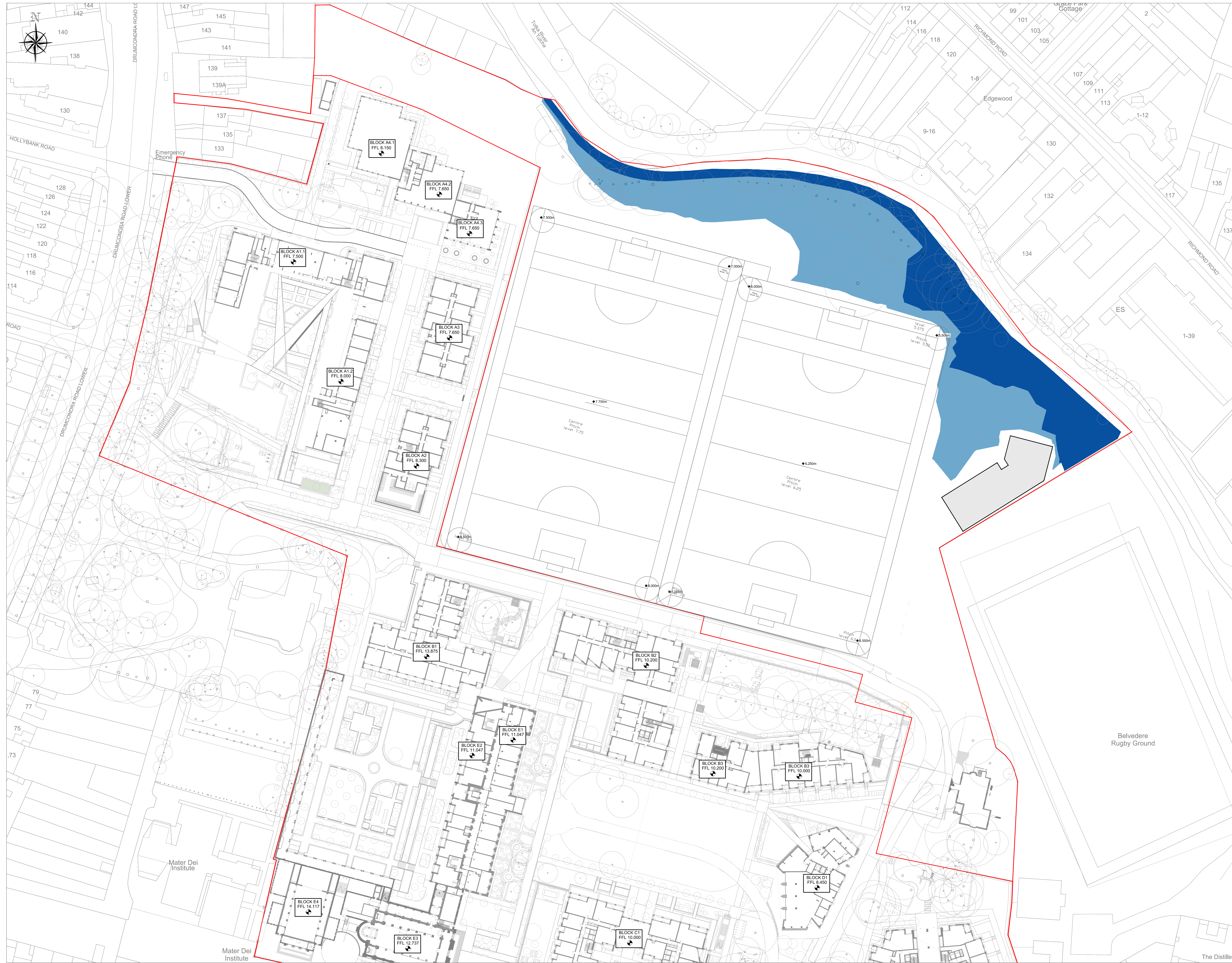
FLUVIAL FLOOD EXTENTS AS PER TOPOGRAPHICAL & PROPOSED LEVELS INFORMATION (OPTION 1) SCALE @ A0: 1:250 SCALE @ A2: 1:500
